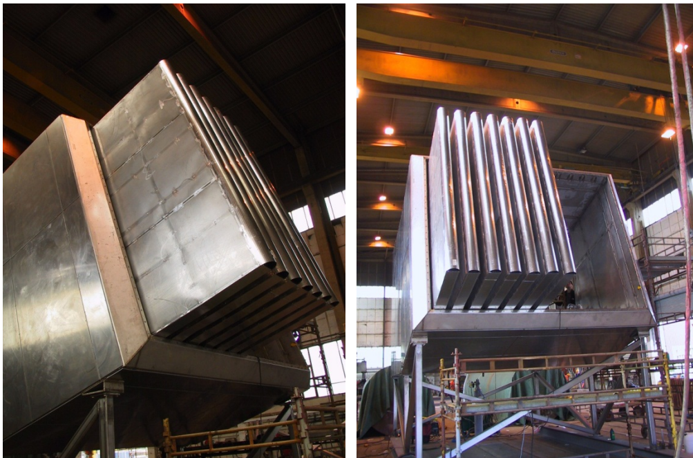
Primary air inlet silencer – PGT25+ gas turbine – Grane
