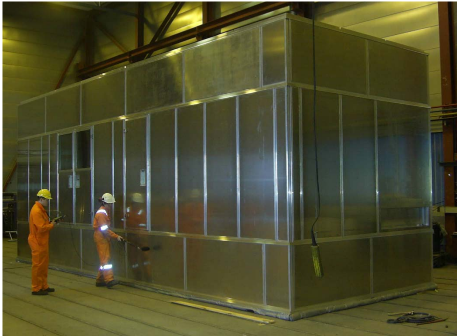
Off base panel noise hood - noise test in our workshop
