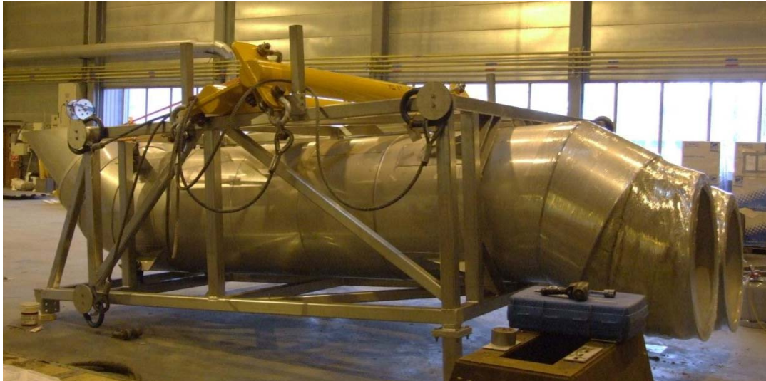
BP Valhall VRD – lifting tools for lifting from ship to platform
