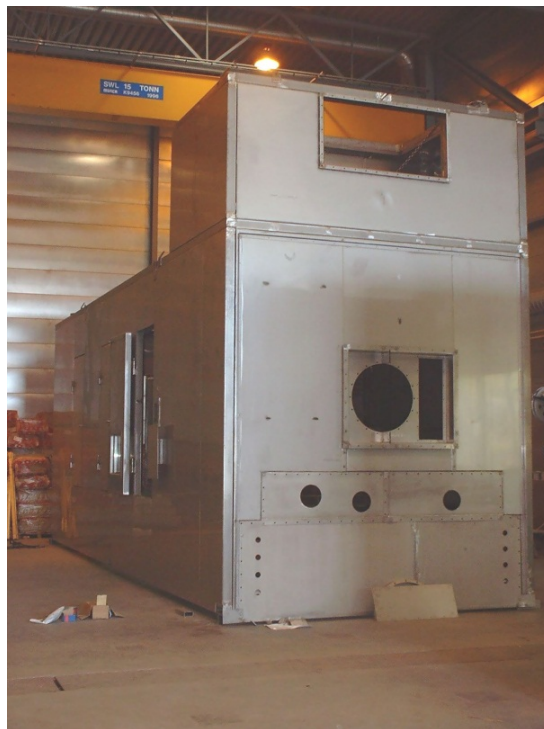
Dan FG - off base noise hood w/atex plenum around exhaust outlet in roof
