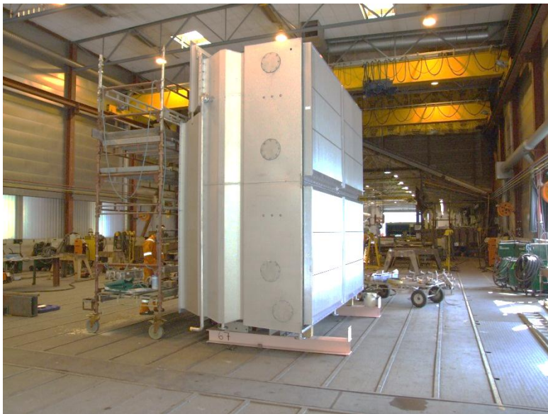
Sleipner T – new filter house in our workshop ready for delivery
