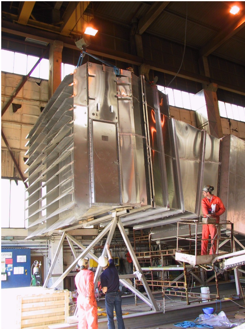
Grane – PGT25+ filter house
