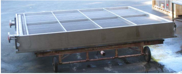
Radiator - liquid media in heat exchanger for Sleipner T.
